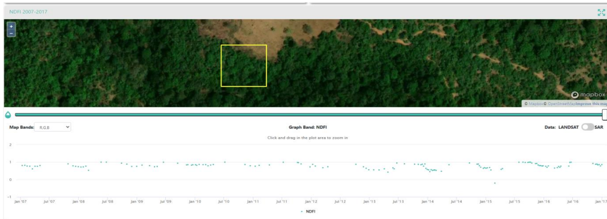
Figure 7: Collect Earth interface for data collection and Google Earth Engine platform for enabling time series imagery for sample plots using Landsat, MODIS and other available imageries.
